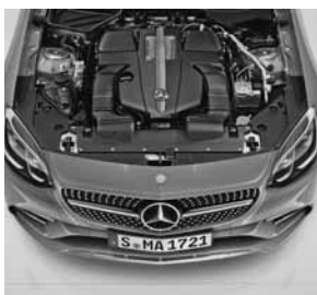
Motor de 3,0 litros V6 biturbo
